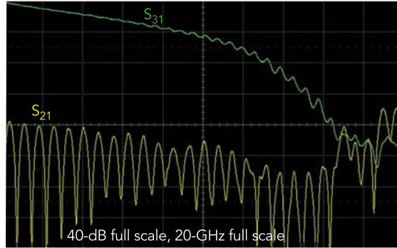
FIGURE 4. The measured S_{21} and S_{31} matrix elements for two stripline traces show that the S_{31} element is clearly an insertion loss, confirming that the case 2 port-labeling scheme was used for this S-parameter matrix.
